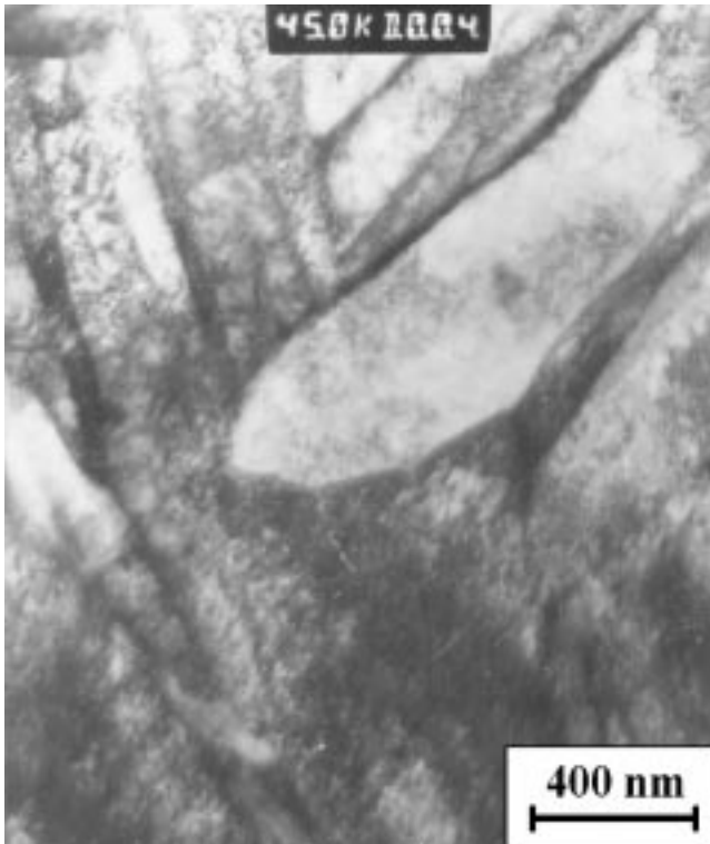
Fig. 5 TEM of heat-treated GPQ sample (900 °C 1 h/WQ/aged at 250 °C)
