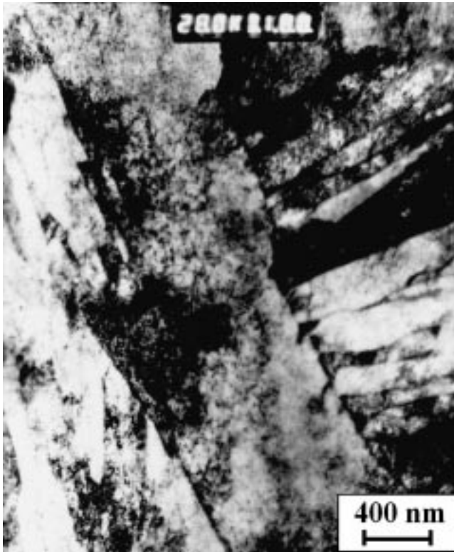
Fig. 4 TEM of heat-treated GRV sample (900 °C solutionized/WQ)
